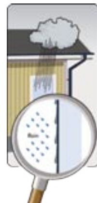
FIGURE 3: Rain washes dirt away. Water droplets spread out to form a 'sheet', dirt particles on surface are picked up by water and washed off glass.
