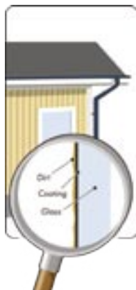
FIGURE 1: Coating is activated by UV light. After installation the special coating needs 5 to 7 days exposure to daylight to activate.
