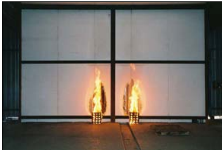
Figure B3-2: Material deforming up to purlin on both sides (t = 5 min)
