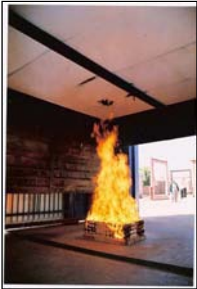
Figure B1-2: Material deforming and opening up in area above heat source (t = 4 min)
