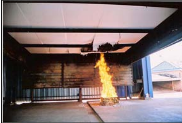
Figure B1-3: Larger area above fire source damaged but no ignition (t = 8 min)
