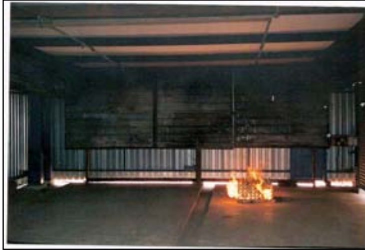
Figure B2-1: Test installation shortly after ignition of ignition source
