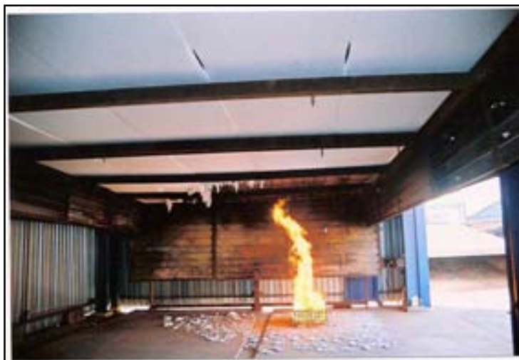
Figure B1-4: Fire source decaying – no further spread of damage to installation (t = 15 min)
