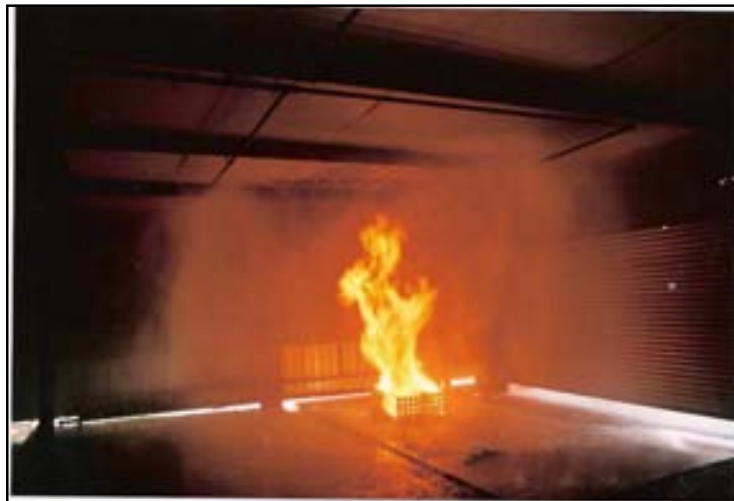
Figure B2-4: Second sprinkler activated, no further damage to test installation (t = 9 min 30 s)
